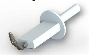
This precision-engineered jointed finger probe is manufactured in full compliance with the IEC standards listed below and is also recognized for use in both Canadian and U.S. standards. Designed to simulate the movement and reach of a human hand, it features a palm simulator and restricted joint articulation to mimic realistic touch and access.
