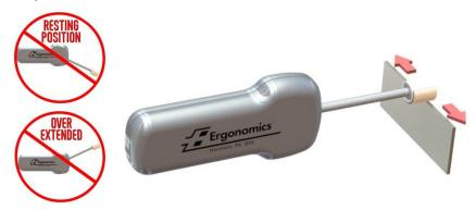
Maintain the proper pressure while moving side to side along the surface to be tested. Most standards suggest that 100 mm (about 4) inches) increments be investigated. If a 100 mm sample is not available, the same surface can be used repeatedly until the proper length is investigated. 100 mm in total length is not to be exceeded for a normal test. Consult the applicable standards for the exact requirement.
